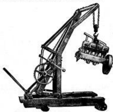
As a Portable Floor Crane for Inside or Outside Uses. Capacity, 1½ Tons. List Price $137.50.
