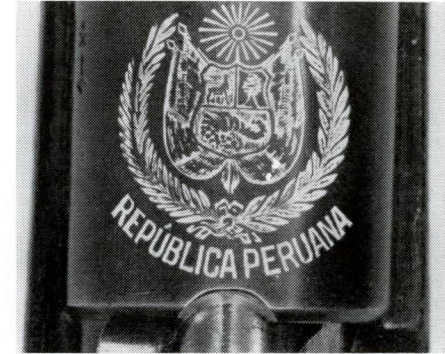
Peruvian Model 1935 .30-'06 short rifles bear the Peruvian coat of arms, and the left of the receiver denotes manufacture in Belgium by FN. Circular cut on rear of receiver ring gives loading clearance for .30-'06 cartridge which is longer than 7 mm., 7.65 mm., and 7.9 mm. Mauser cartridges, the most common Mauser military rounds.
