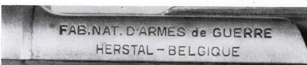
Marking on receiver wall of Venezuelan Model 1924/30 7 mm. short rifle denotes manufacture by Fabrique Nationale D'Armes de Guerre (National Factory For Military Arms), abbreviated FN, Herstal, Belgium.
