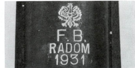
Polish Mausers bear the Polish eagle coat of arms. The "F.B. RADOM" marking on a Model 29 7.9 mm. short rifle stands for Fabryka Broni Radom (Radom Arms Factory). "1931" is the year of manufacture.
