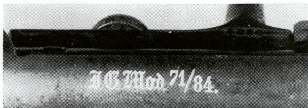
"I.G." in marking on German Model 1871/84 11 mm. Mauser blackpowder rifle stands for Infanterie Gewehr (Infantry Rifle).
