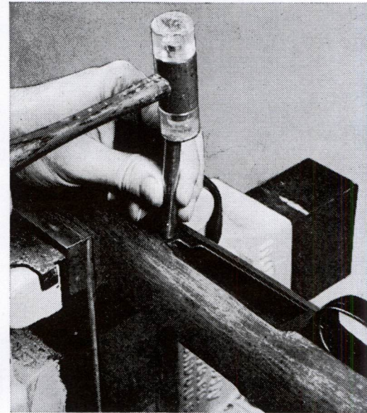
6 Trigger guard is inletted first. Film of spotting color is applied to bottom and sides of guard which is then tapped lightly into its mortise. This transfers spotting color to tight spots which must then be pared and scraped away with flat chisel and penknife blade. Many impressions are required to fully inlet guard, which is knocked out each time by punch through magazine mortise.
