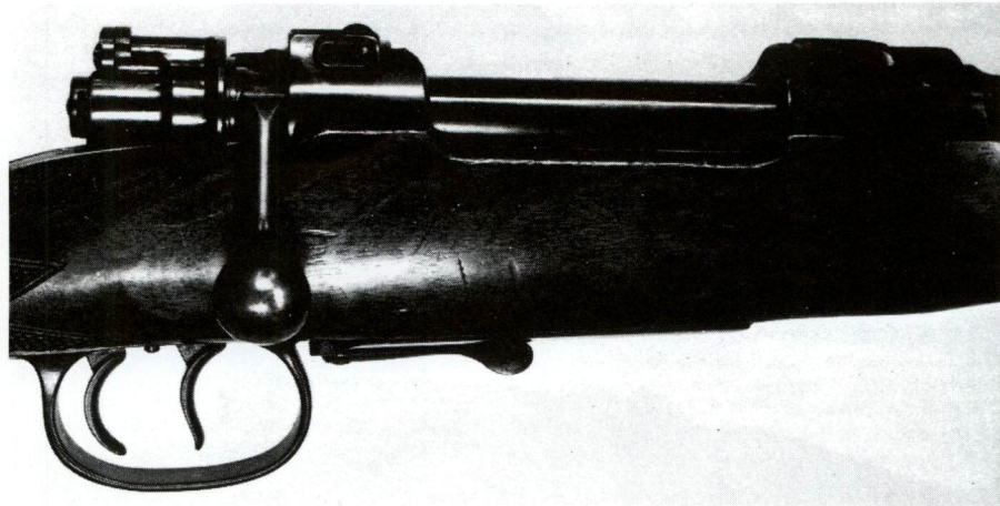
Oberndorf Mauser sporting rifles were made in many styles and calibers. Specimen shown is chambered for 8x57 Mauser cartridge and is equipped with double set triggers. Donated to NRA Museum by Rev. J. B. M. Frederick.
