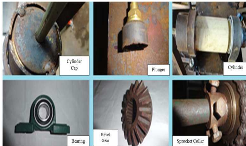
Figure 2: Some of the Parts Fabricated and Used for Assembling the Pump Set
